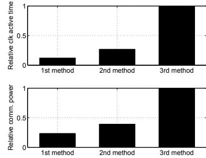
Fig. 6. Relative clock active time and communication power consumption for the three inter-processor communication methods described in Fig. 5 for a 2-D  $8 \times 8$  DCT application
