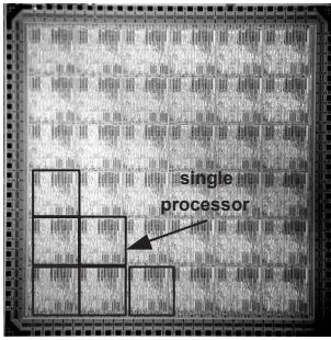
Fig. 13. Chip micrograph of a  $6 \times 6$  GALS array processor [5]
