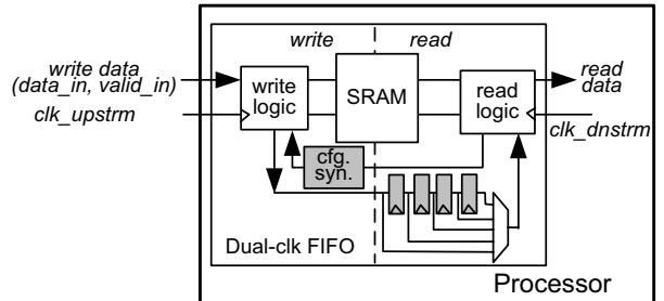
Fig. 4. Configurable logic at the asynchronous boundary in a FIFO; two clock domains exist within a single processor
