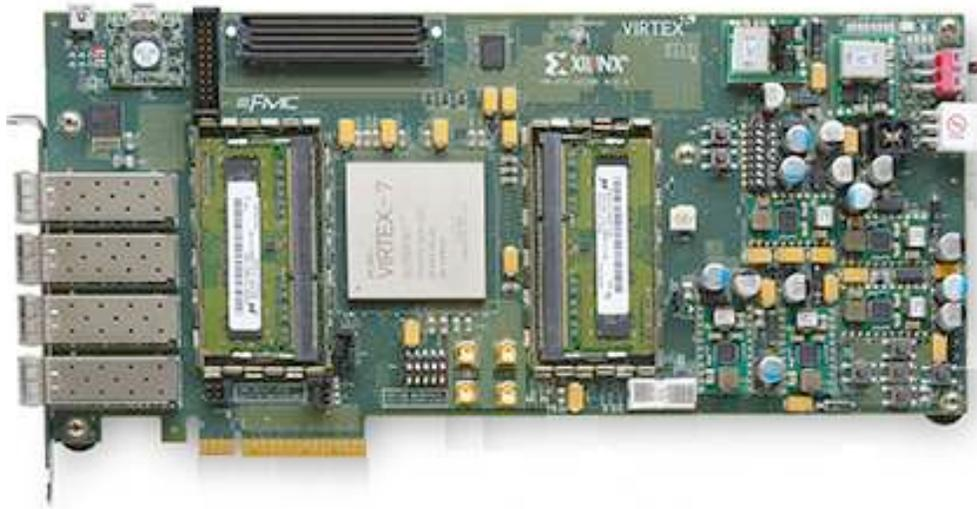
Figure 4.1: The Xilinx Virtex-7 FPGA VC709 Connectivity Kit
