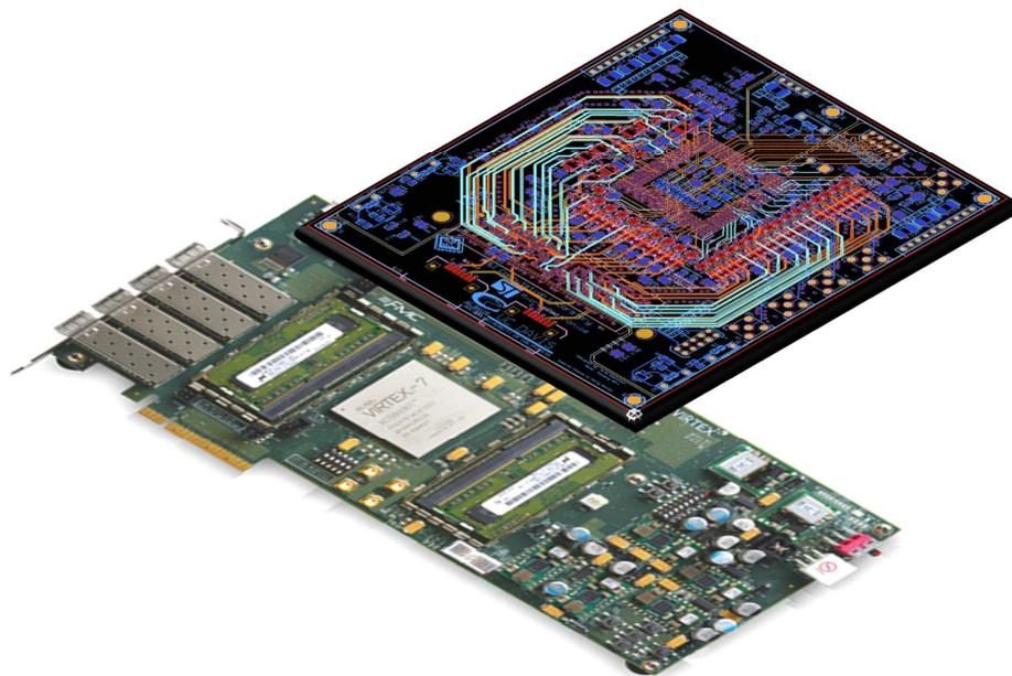
Figure 1.3: A physical view of the designed Picoblade with a layout view of the daughter card
